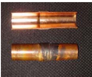
Charge N2 to the pipes
