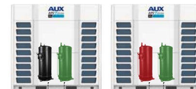
Running Backup compressor start up Failure
